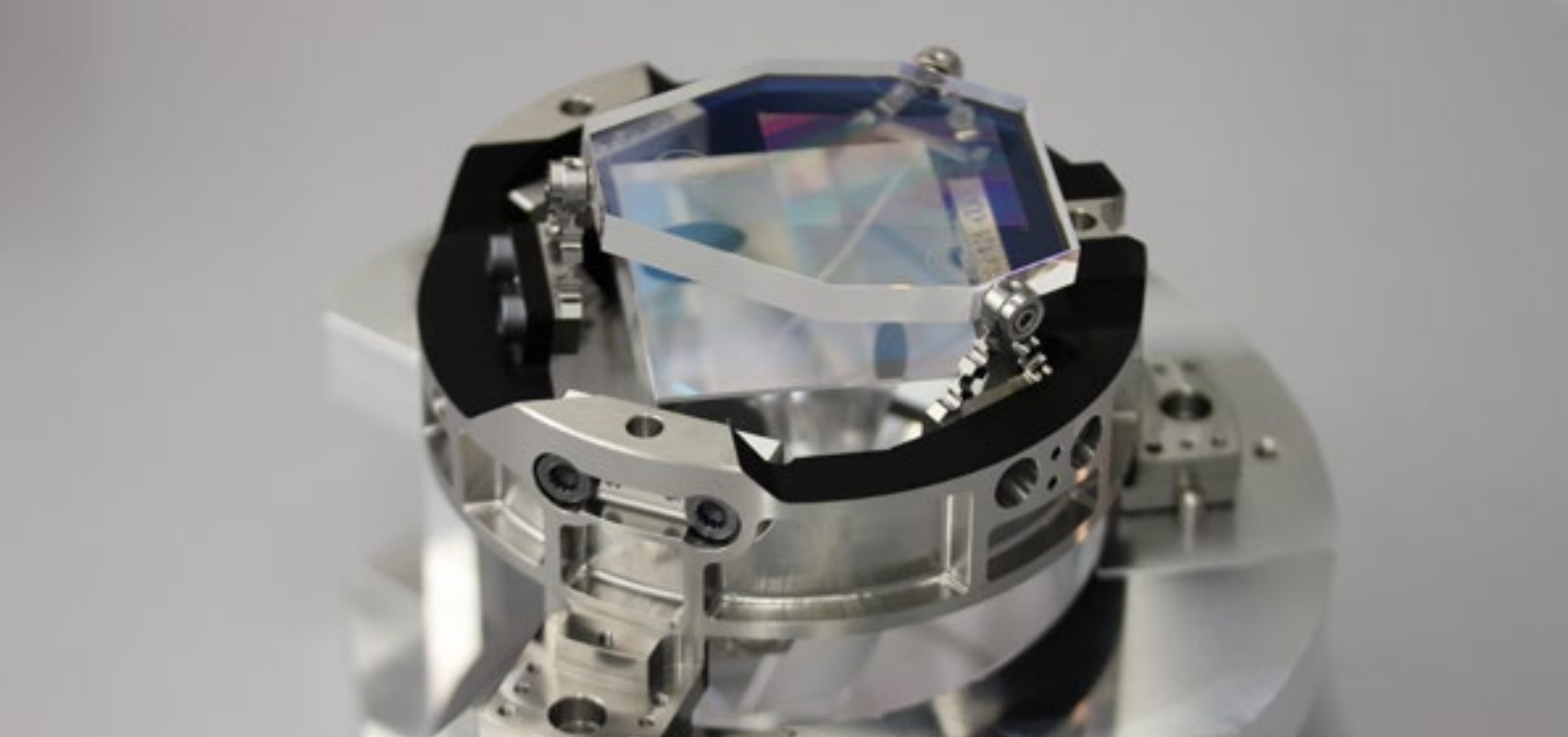
[1] Prism-Grating-Assembly für Sentinel 5 (Flughardware). / Prism Grating Assembly for Sentinel 5 (flight hardware)
